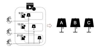
Luminaires not included in a condition scene will trigger to an earlier valid condition state (e.g., All 3 lamps ON in the last condition)
