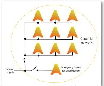
Emergency scene will only be active when power is ON to the Emergency Smart Switched device
